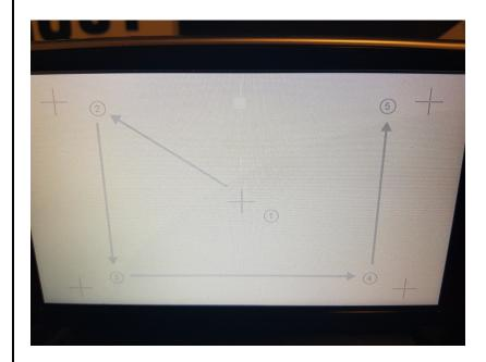
If the unit is stuck on the calibration screen, you will need to calibrate it correctly in order to exit from this screen.
