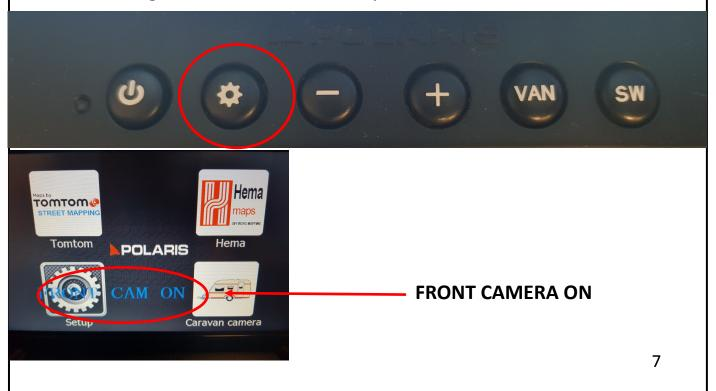
Press the minus button to change the setting to FRONT CAMERA OFF
