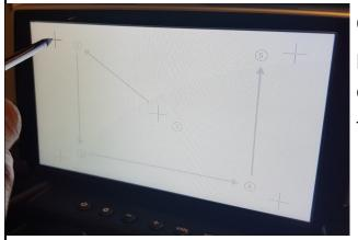
Once you have the appropriate tool, please hold your tool down on the centre of the cross. The cross will move around the screen automatically
