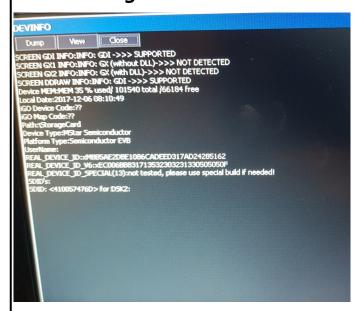
This is an easy fix, it just means that the NAV path file is set incorrectly and has been set to \StorageCard\DeviceInfoDig.exe
