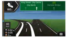
**Cause**: If you are approaching a motorway exit or a complex intersection and the needed information exists, the map is replaced with a 3D view of the junction. The lanes you need to take are displayed with arrows.
