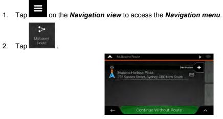
3. There is only one line in the list of route points, the starting point of the route, which is normally the current GPS position.
