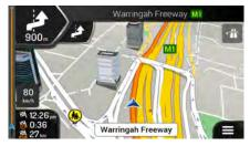
There is a field in the top left corner displaying the next manoeuvre. Both the type of the manoeuvre (turn, roundabout, exiting motorway, and so on) and its distance from the current position are displayed.
