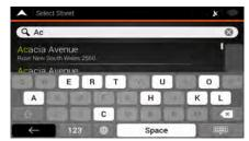
**Cause**: Hilux navigation has a smart keyboard for address search, which means that only those buttons are active that can be used to type a name that is available on the map.
