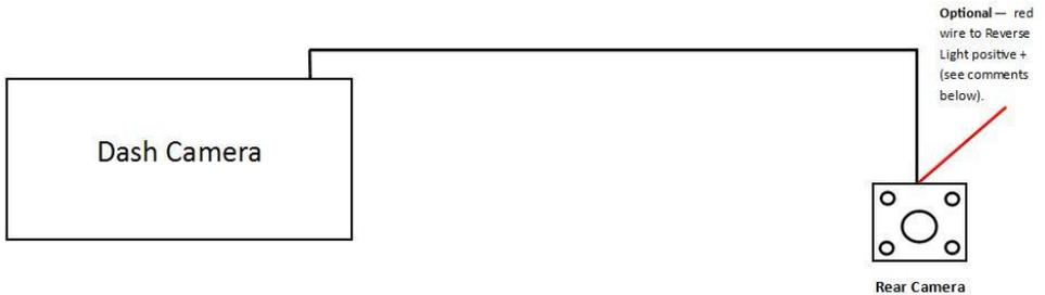
1. Rear camera receives power from the dash camera when plugged in. You do not have to wire up the red wire to power up the rear camera for recording purposes.
