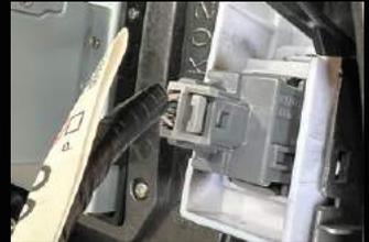
Remount the switch into the fascia panel & don't forget to plug the cable back in for the Hazard switch.
