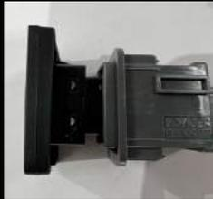
Release the keyways to release the OEM Hazard switch.
