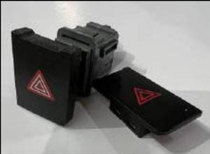
New hazard switch is located in the satchel bag with all of the cables
