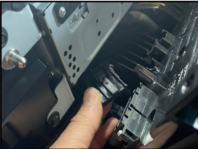
3. Remove all plugs from the back of the air conditioning control panel, remove trim and set aside
