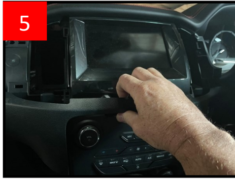
5. Place your hand on the long trim directly underneath the monitor and loosen by popping out carefully
