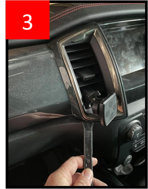
3. Put trim tool under left of OEM screen air vent and pop out
