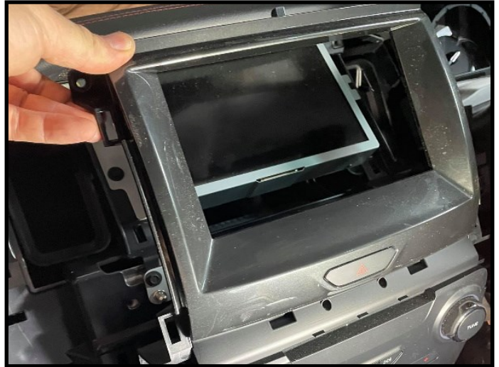
2. Pull the trim off starting at the BOTTOM . Pull gently as you will need to disconnect the plugs from the back of the air conditioning panel
