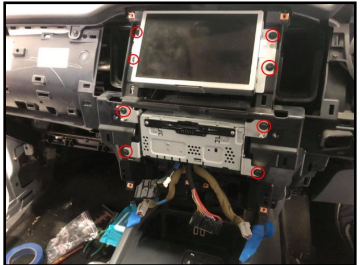
4. Remove 8 screws to access the back of the monitor and head unit
