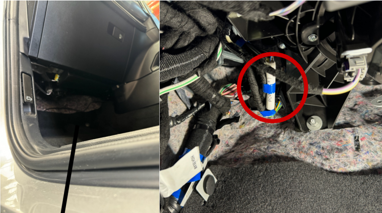
Camera wires are located underneath glove box
