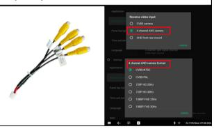
You **CAN NOT** use a CVBS camera as a reverse camera while using an AHD camera as a second camera. The second camera must also be CVBS. Alternatively, both cameras can also be AHD.
